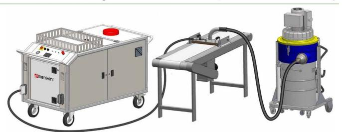
Steam is applied directly onto the belt surface. On impact with the conveyor belt, dry steam easily removes biofilm and product residue. Therefore all product residue and condensation is contained. Debris is removed by the integrated vacuum chamber, which leaves a dry and clean surface. Vacuum chamber is separated by squeegee ensuring that steam hits the belt first and liquidises product. After the cleaning process belt will be allergen-free and sanitised.
